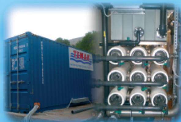
MUNICIPALITY CAPACITY: 1.000 m 3 /day FEED WATER QUALITY: SEA WATER PRODUCT WATER QUALITY: POTABLE
